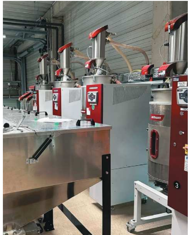
The CMS includes Drymax material dryers.
