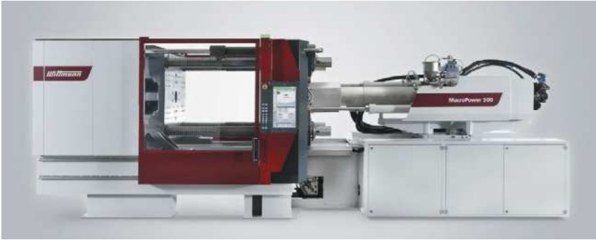
New MacroPower 500/3400 with one-piece machine body. Pictures: WITTMANN
