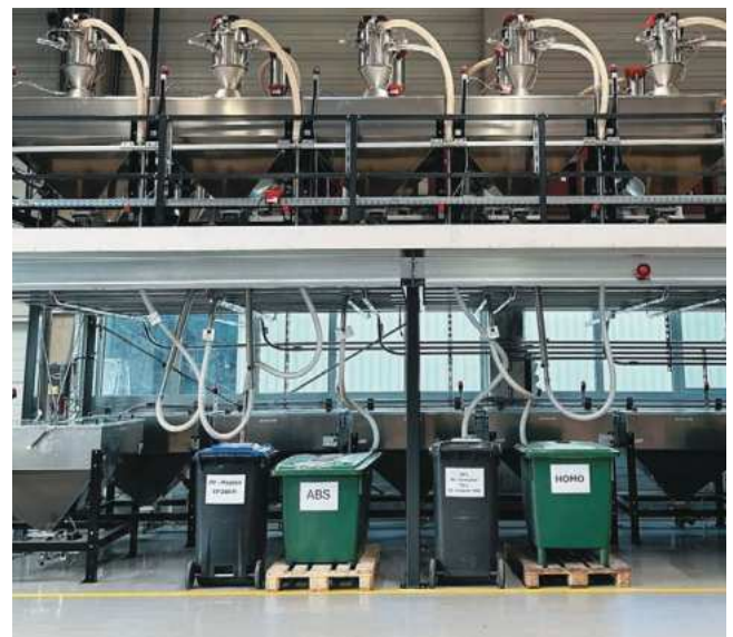
The dryer platform provides a view across the material storage area. The space directly under the platform is reserved for containers filled with the most frequently used materials.
