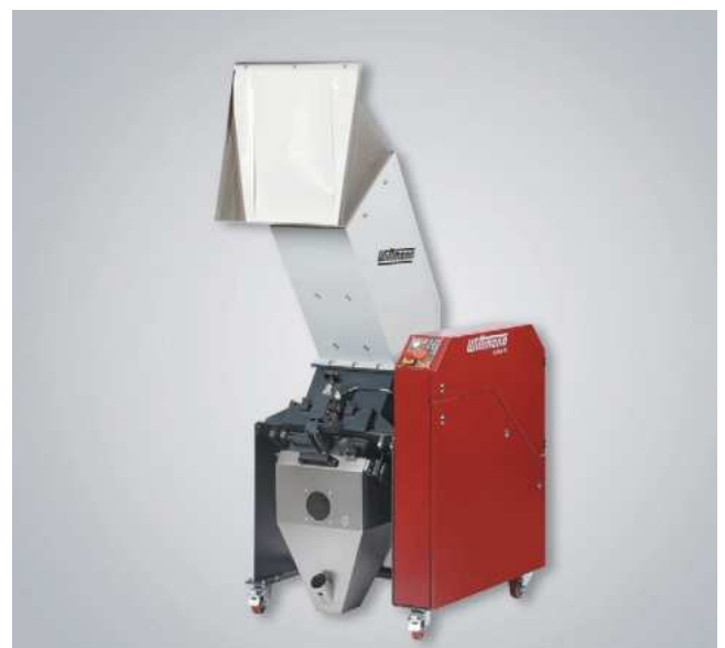
In-house recycling made easy: The G-Max XL granulator is designed for a throughput of up to 100 kilograms per hour.
