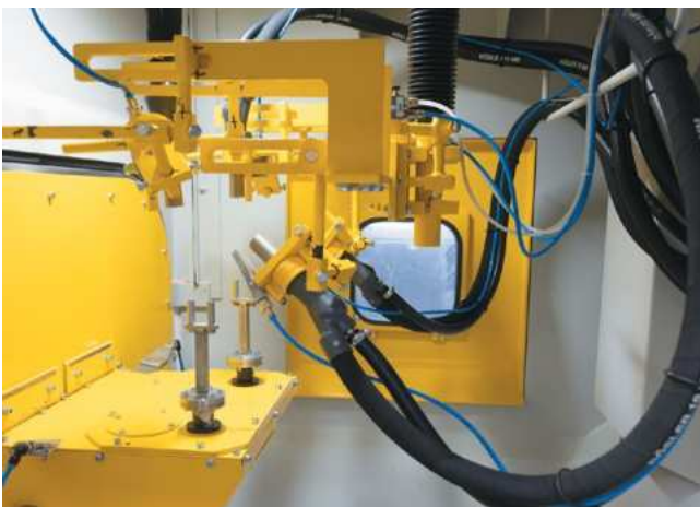
The blast nozzles, placed at the top and bottom of a vertical linear shuttle unit, can be moved up/down and individually turned on or off.
