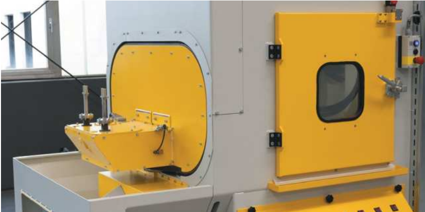
The clever design of the RWS 1200-I4-SAT2 de-flashing system with 2 x 2 satellite stations allows de-flashing work pieces in one chamber, while finished/raw work pieces are unloaded/loaded in another chamber. This greatly minimizes unproductive, idle production times
