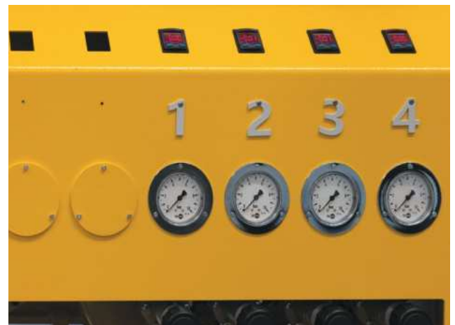
The digital pressure control of each individual nozzle ensures high process safety and stability (all images: Rösler)
